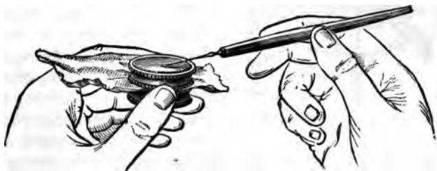
FIG. 240.—Drum Used to Test the Cutting-Edges of Eye Instruments.
